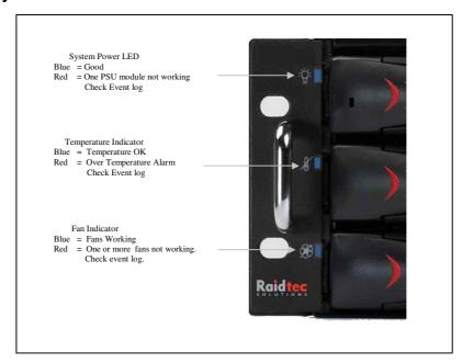
Figure 5-3 – System Indicator LEDs
